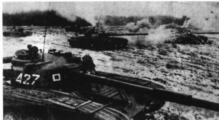
The initial production of the T-64 with D-81T gun lacked a thermal sleeve over the gun tube. This vehicle can also be distinguished by the right fender ZIP tool storage bin on the fender.
