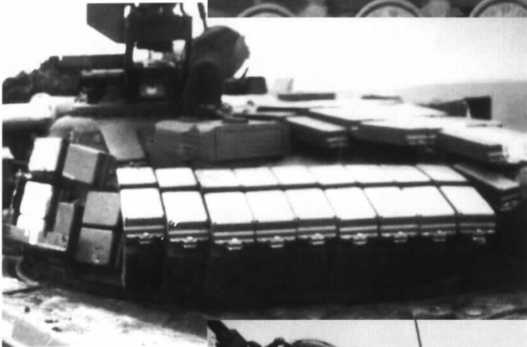
A close-up of a T-64BV turret, also showing the Kobra control box.
