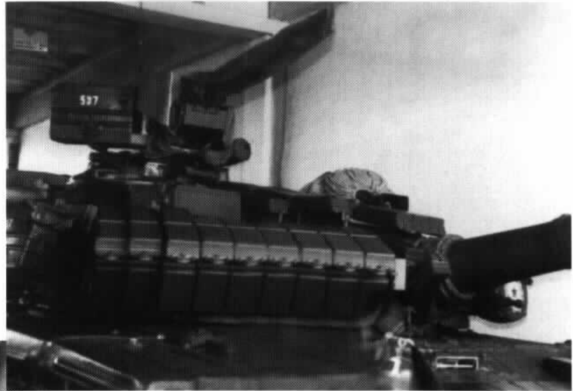
A frontal view of a T-64BV showing the arrangement of the ERA bricks. This view is also interesting in that it shows the Kobra control box.
