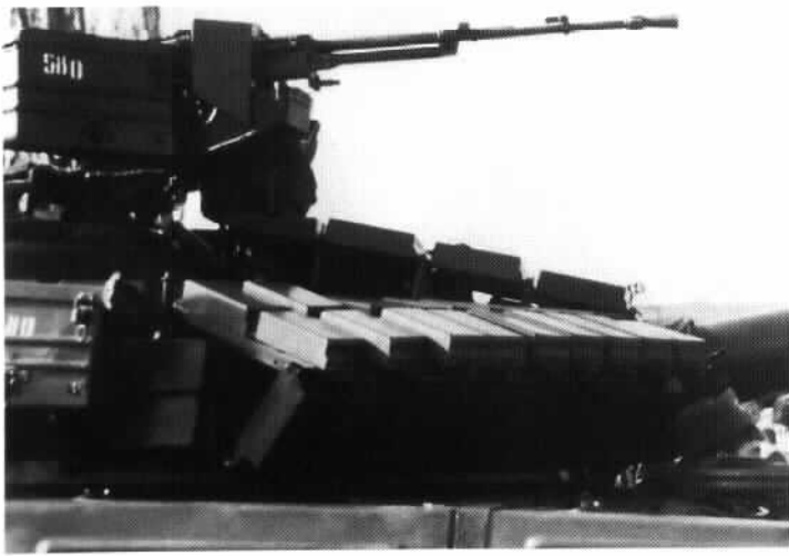
A T-64BV showing the ERA brick arrangement. Notice how far the roof bricks are spaced from the turret roof. Also note that the final row of bricks in the array are of a different cross-sectional shape.
