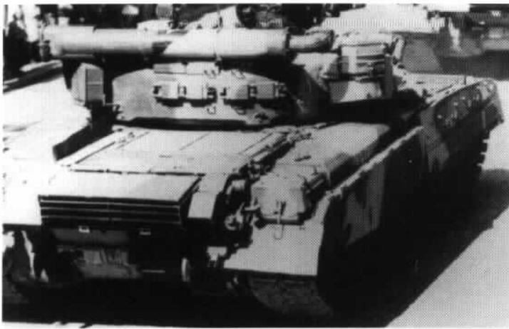
A rear view of the T-80U. Under the grill is additional track stowage.
