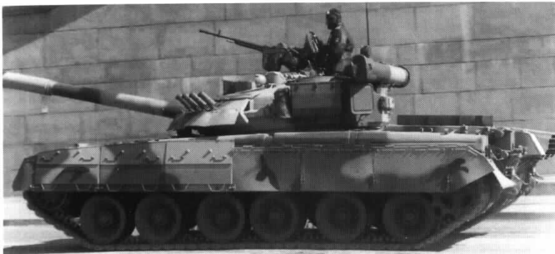
Another side view of the T-80U moving into position in Moscow for a Kremlin parade. The T-80U is not fitted with the usual rear stowage bracket for the OPVT snorkel seen on the earlier T-80B.
