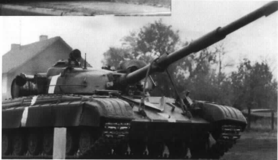
Another T-64A rebuild during summer exercises. This vehicle is an older T-64 with the initial gun-tube minus the thermal sleeve, turret grab-iron and fender ZIP boxes.
