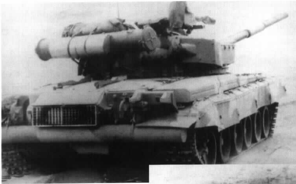
A rear view of the T-80. The T-80 turbine engine requires a large exhaust port at the rear. The engine air intake is immediately behind the turret.
