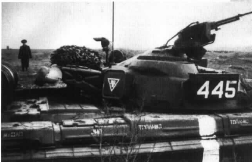
An overhead view of a T-64B tank. This variant had a new turret of slightly different shape on the front. In addition, the turret had a layer of plastic anti-radiation liner added over the top of the roof and the rear of the turret. The main feature of this variant was the addition of a guidance control box for the Kobra missile in front of the commander's station, obscured by the commander's NVST machine gun in this view.
