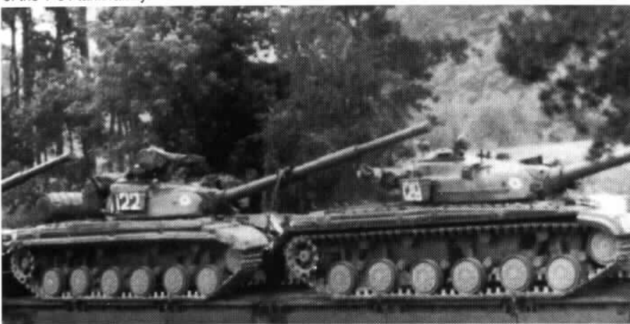
A pair of T-64A in transit with a regimental unit insignia evident on the turret front-two concentric circles with the inner circle having a hollow triangle. The lead vehicle is an early production T-64 with the fender mounted ZIP stowage bin. Another feature of this variant is evident here- the long grab-bar at the base of the front turret sides. This feature was dropped on the standard T-64A.
