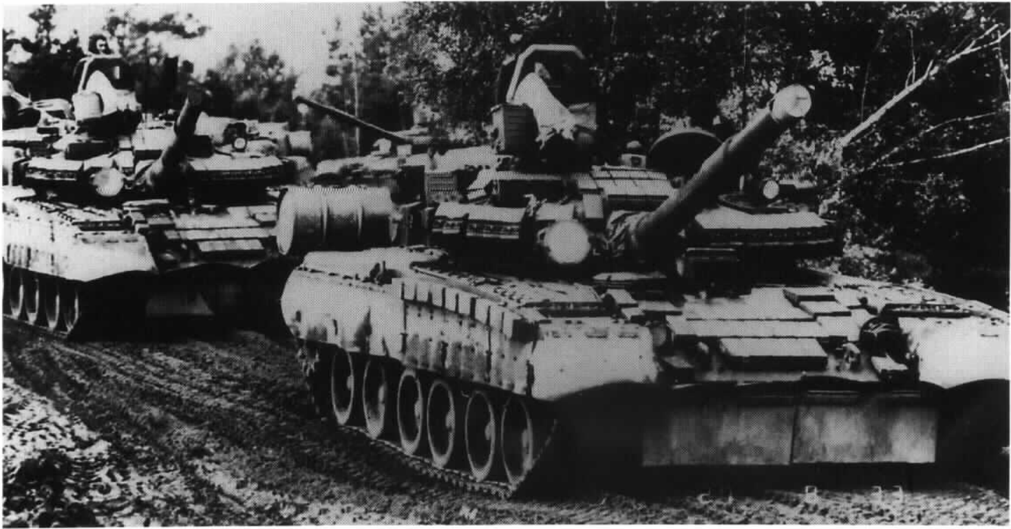
A company of T-80BV on the move. The lead vehicle has a partial array of ERA bricks on the side panels.
