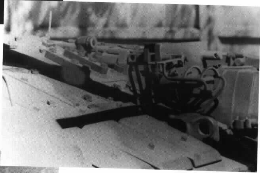
A detail shot of the complicated protective covers over the searchlights on the T-80U.
