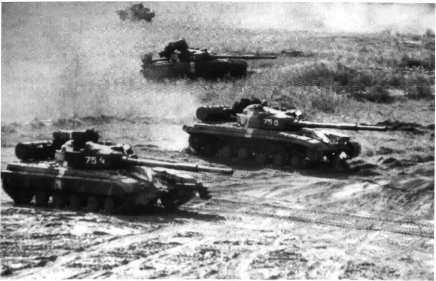
Summer wargames in the late 1980s, with a T-64A fitted with KMT-6 mine rakes.
