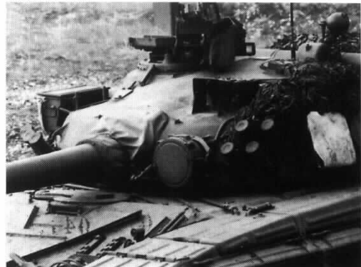
A detailed front view of a T-64B turret. The most distinctive feature of this variant is the enlarged gunner's sight which contains a laser rangefinder. Also evident in front of the commander's cupola is wiring leading down to where the Kobra control box is fitted-the box is not present in this view. The other characteristic of the T-64B-the new turret, is a more subtle change, noticeable by the slight plateau effect of the front edge of the turret roof. The T-64B also carry fewer smoke grenade launchers than the rebuilt T-64A.
