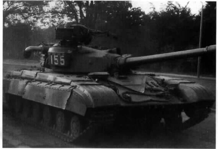
The T-64A (rebuild) is an upgraded T-64 or T-64A. The hull glacis plate has an added layer of about 30mm of steel armor applique added. This can be most easily determined by the reduction of splash strips in front of the driver. Normally there are four, after the upgrade there are only two. Other internal improvements probably took place at the same time on the vehicle's transmission.
