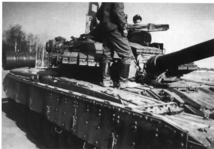
A good close-up of the T-80BV side skirts. The many small bolts are used for the attachment of ERA bricks.
