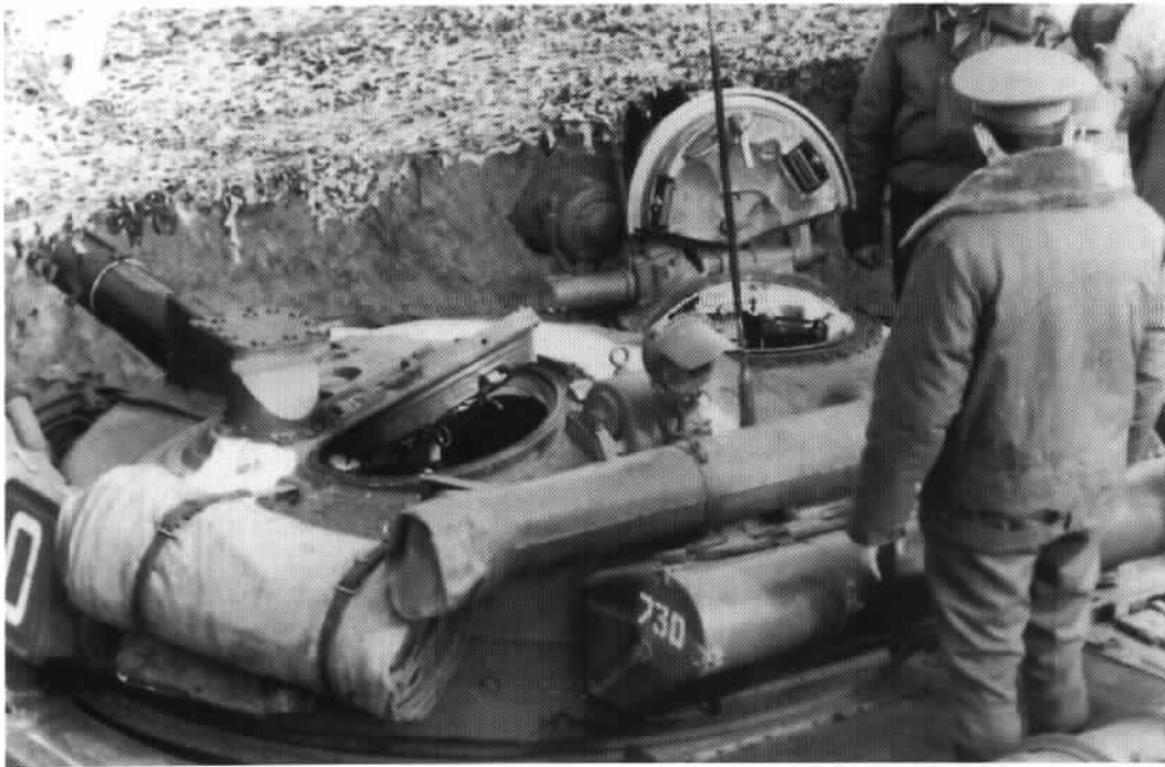
A close-up of the turret of a T-64B. The later production T-64B (possibly the T-64B1 series), had additional plastic anti-radiation liner added to the turret roof and the turret rear sides. This can be seen by carefully studying the photo-the small circular plugs characteristic of this material are evident.
