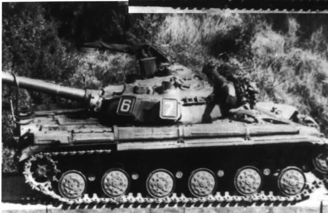
A heavily stowed T-64A with the Central Group of Forces in Czechoslovakia in the 1980s. It lacks the full OPVT tube stowage.
