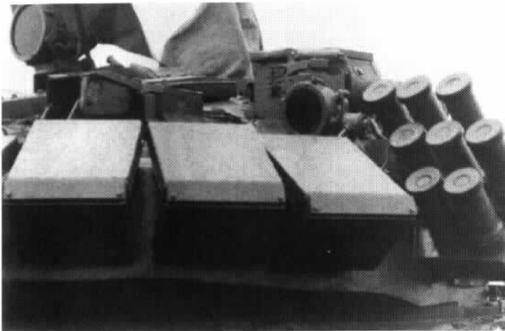
In 1990, some T-72B1s began to be fitted with the 2nd generation reactive armor first seen on the T-80U. This version also has the 1K13 laser sight, evident above and behind the smoke mortars. This version is called SMT M1990 by NATO, but its Soviet designation is not yet certain.
