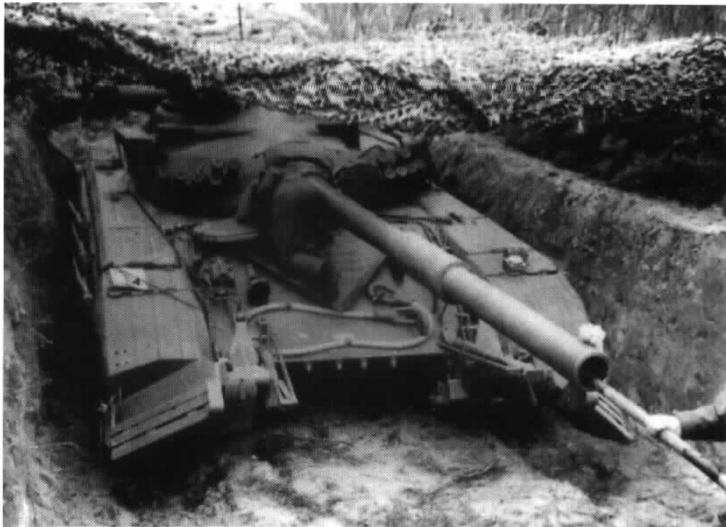
A T-64A having its bore cleaned. This particular tank is fitted with KMT-6 mine rakes.
