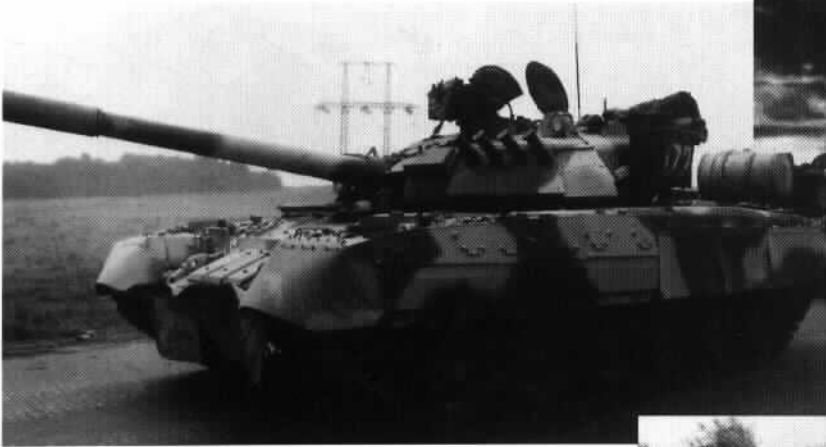
A rare view showing the OPVT snorkels in operation on the T-80U. The snorkel configuration on the T-80U is more similar to that on the T-64 than the T-80B.
