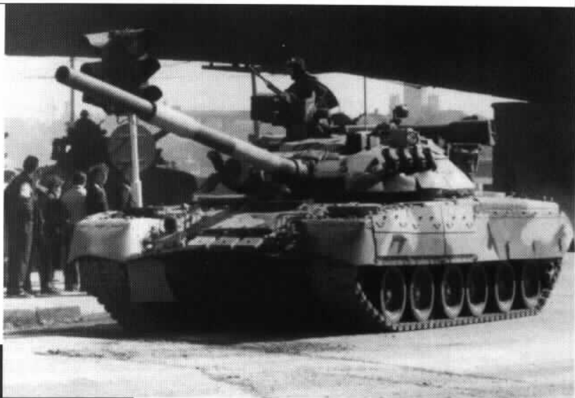
A T-80U of the 4th Guards Kantemirovets Tank Division in Moscow. The new applique armor extends down over the side skirts.
