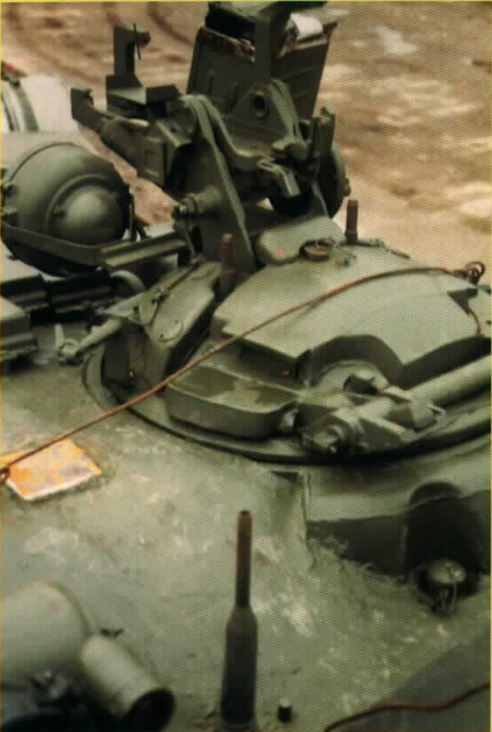
A detail view of the tank commander's cupola, showing the NSVT machine gun mounting minus its weapon. (Michael Jerchel)
