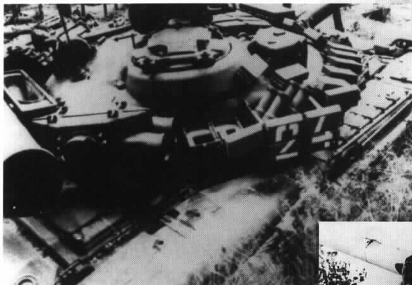
An overhead view of the T-80BV. The large device immediately to the rear and below the commander's cupola is a pair of covers fitted over the engine air intake. These covers have tubes which are then attached to a pair of OPVT wading snorkels.
