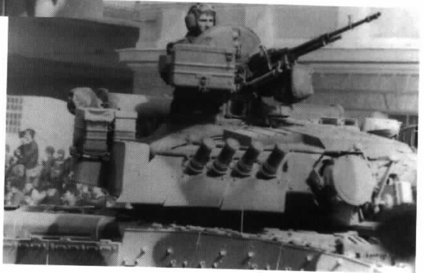
This view clearly shows the similarity between the T-80U's machine-gun mounting and that of the older T-64, right down to the larger ammunition box. Two spare ammunition boxes are carried further to the rear on the turret side.
