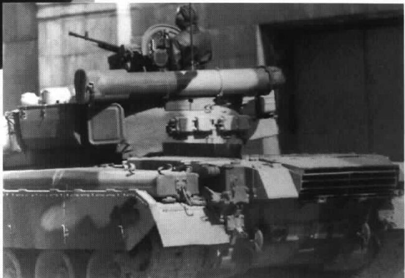
Although a bit murky, this shot shows the attachment brackets for the unditching beam underneath the engine exhaust grill. The beam is not present in this view.
