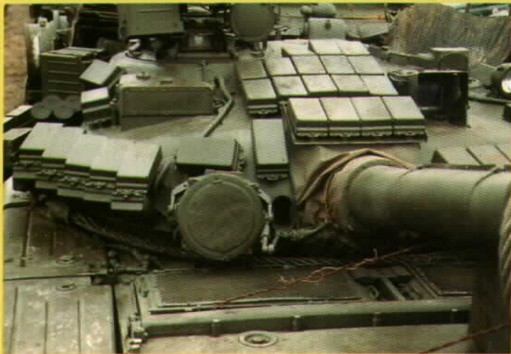
An overall view of the right turret side of a T-80BV showing the layout of the reactive armor bricks. In this view, the turret is pointed rearward, so details of the engine deck are also evident. The large screened area immediately under the searchlight is one of two air intakes for the turbine engine. (Michael Jerchel)
