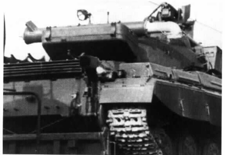
A T-64B on exercise in Hungary in 1989. The small attachment point for the Kobra guided missile control box is evident in front of the commander's cupola.
