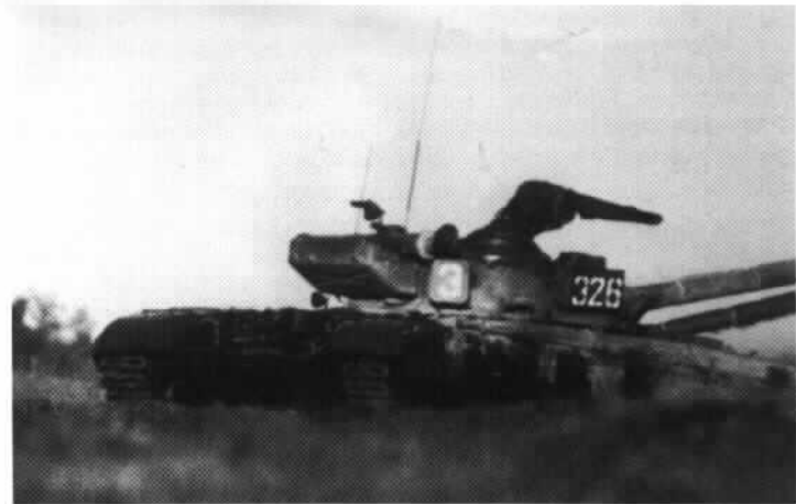
The same tank, bort number "326" with the turret traversed to the rear. This shows some details of the rear stowage bin.
