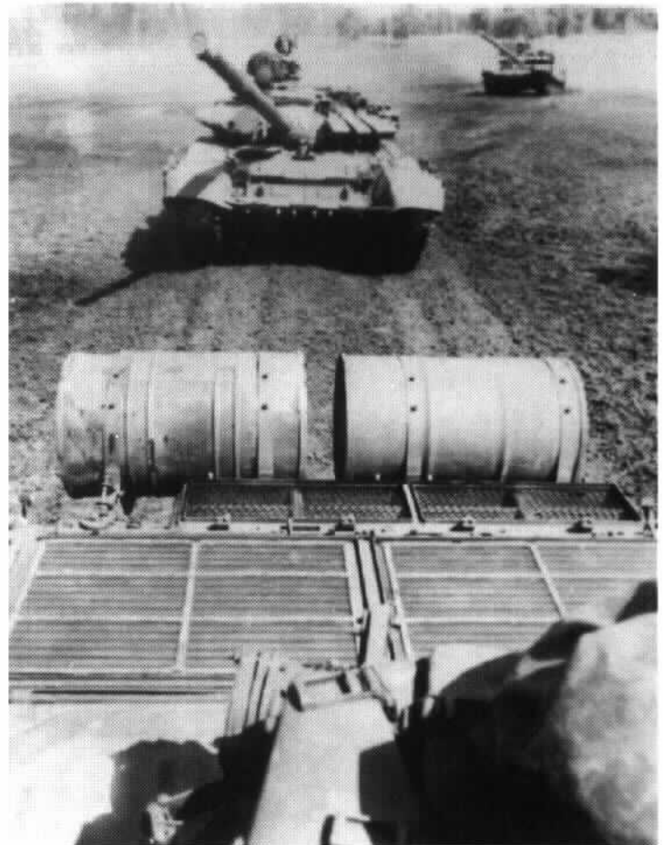
An overhead view of the engine deck of the SMT M1990 which suggests that it is powered by the same V-84 diesel as the T-72B1. In the background are two more of this new tank type.
