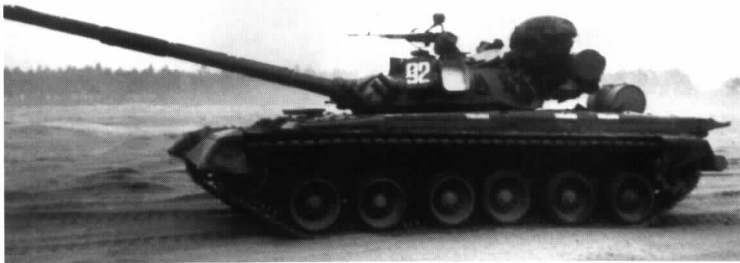
A T-80 on the move, heavily stowed. The characteristic feature of the T-80 is the new roadwheel- larger than a T-64's, smaller than a T-72's. The commander's machine gun cradle is a simple manual type, not the remote control type found on the T-64.
