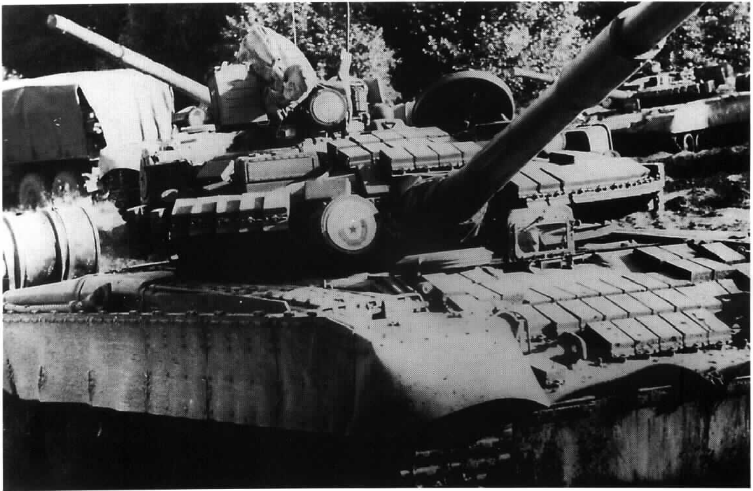
A close-up of a T-80BV. Note that the bricks on the glacis plate are not attached directly to the armor, but space off about an inch.
