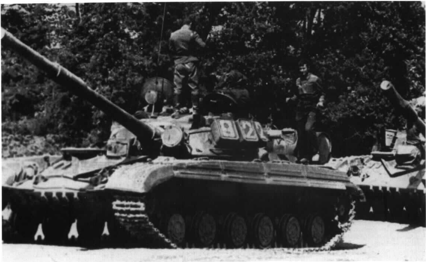
A T-64R still in service in the 1980s. The only distinguishing feature of this variant is the shorter gun tube.
