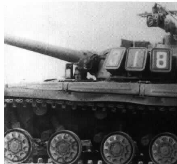
A clear side view of a T-64A showing the method of attaching blocks to the suspension. The blocks are attached to the left, while the racks for two more blocks are attached to the right. Most vehicles have only two racks, located horizontally rather than vertically.
