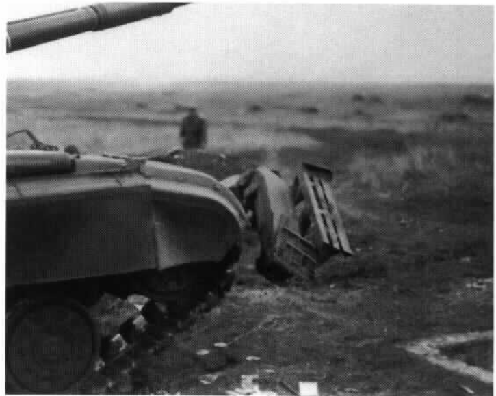
A view of the KMT-6M2 mine rake in the folded (travel) position.
