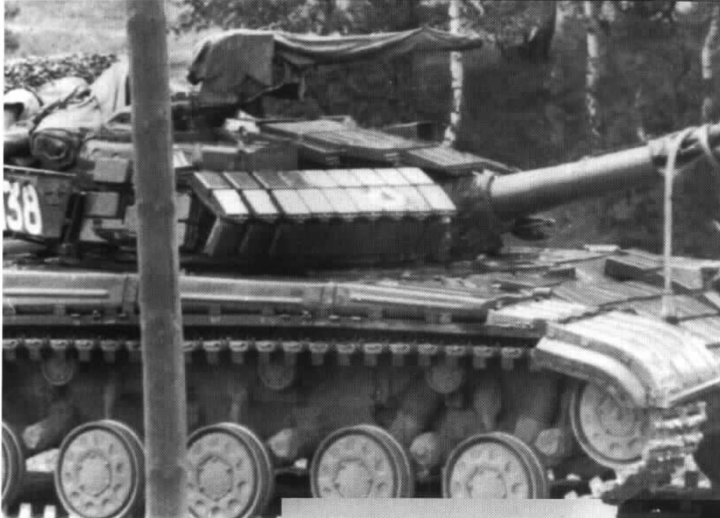
A detail view of a T-64BV showing the frontal ERA brick arrangement.
