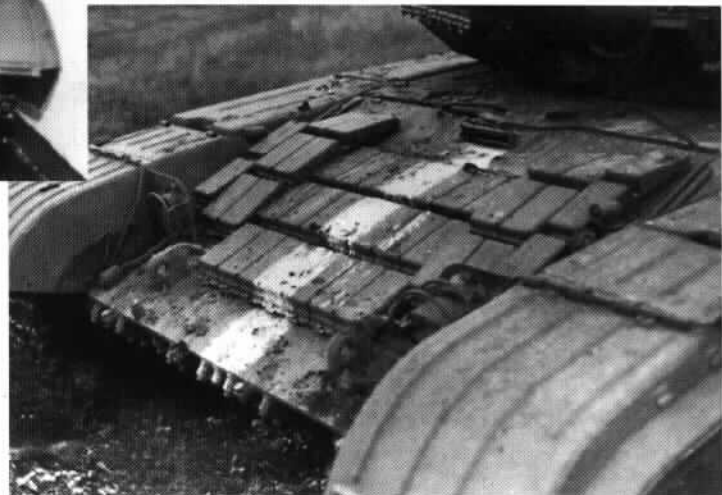
Another frontal view of the T-64BV. This angled view accents the fact that the outer bricks are not fitted flush to the glacis plate. Notice also that the upper row of bricks use the wedge shape rather than the more common brick shape.
