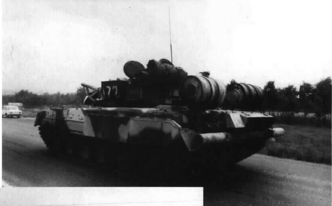
T-80Us on their way to Moscow during the coup. The vehicles have the fuel tanks stowed up on the rear engine deck instead of over the rear fenders as is more commonly the case with turbine powered T-80Bs. (Dr. Udo Bauer Via Thomas Anderson)
