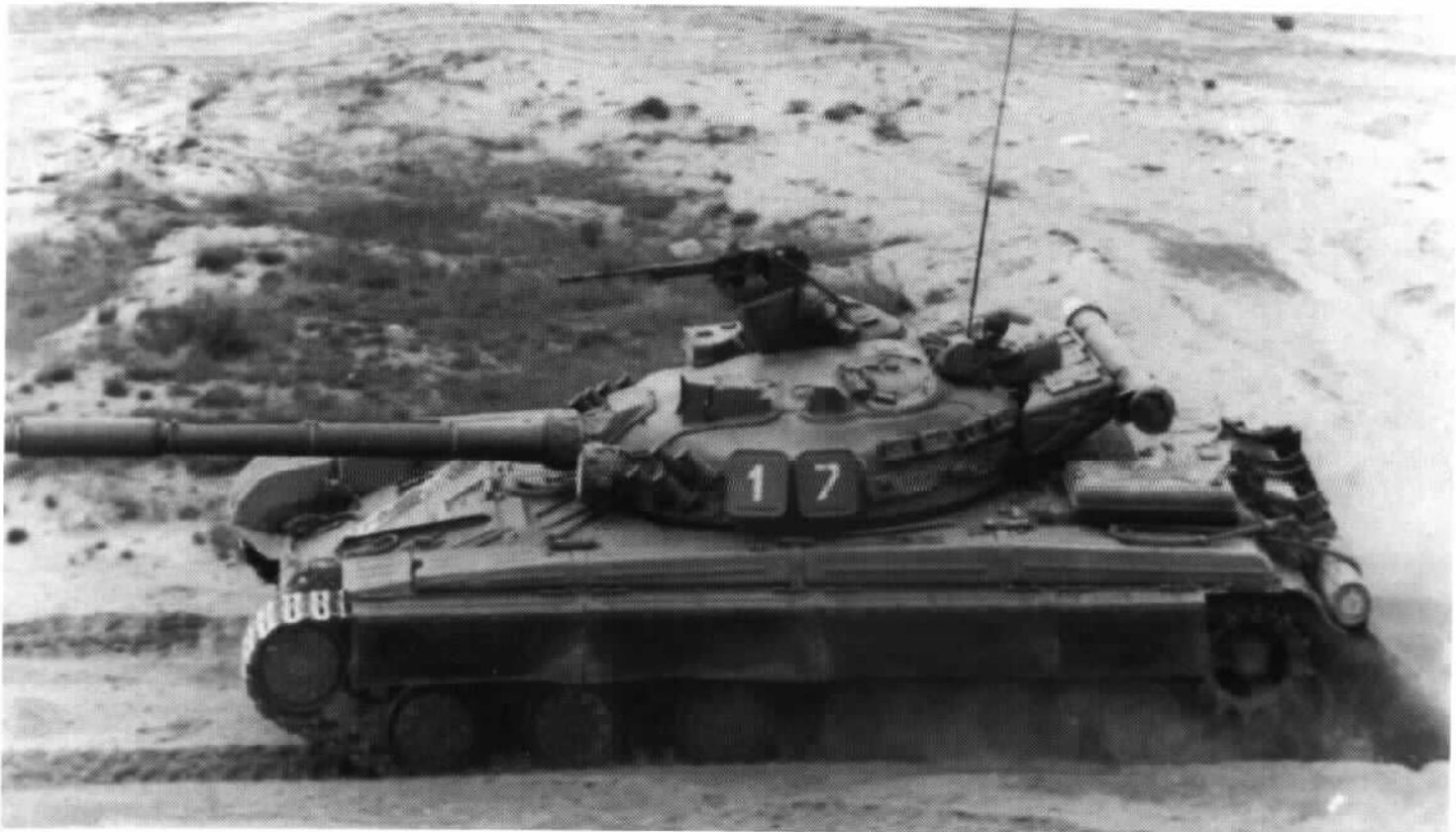
A fine character study of a T-64B on wargame maneuvers in 1989. This vehicle has the Kobra control box fitted in front of the commander's station. The other typical T-64B features are present as well including the increased glacis armor, enlarged gunner's sight, and smoke mortar configuration. Note also the use of a T-55/T-62 fuel pannier instead of the more usual 200 liter drums.
