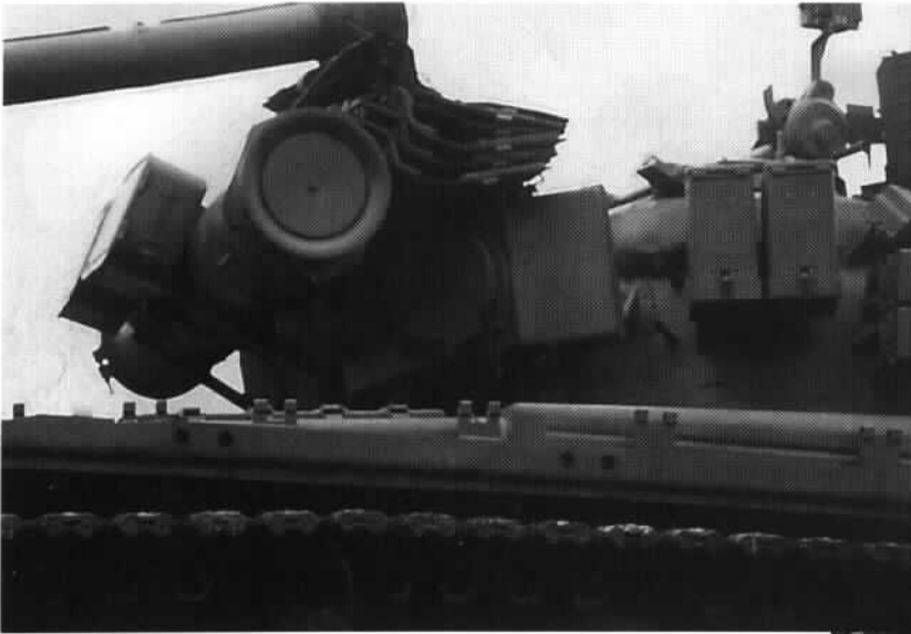
A close-up showing the shock absorber and torsion bar extension on a T-80BV. (Michael Jerchel)
