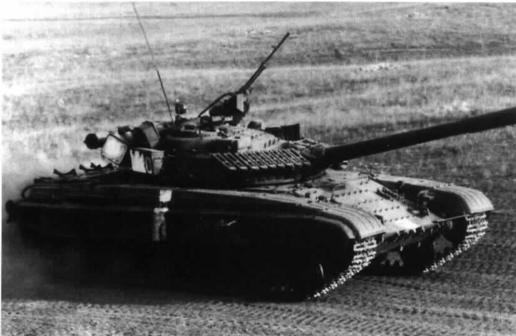
A T-64BV, minus the explosive bricks on summer maneuvers. The many small attachment bolts are very evident in this view. Notice also that the stowage bins and smoke mortar layout has been changed to accommodate the ERA.
