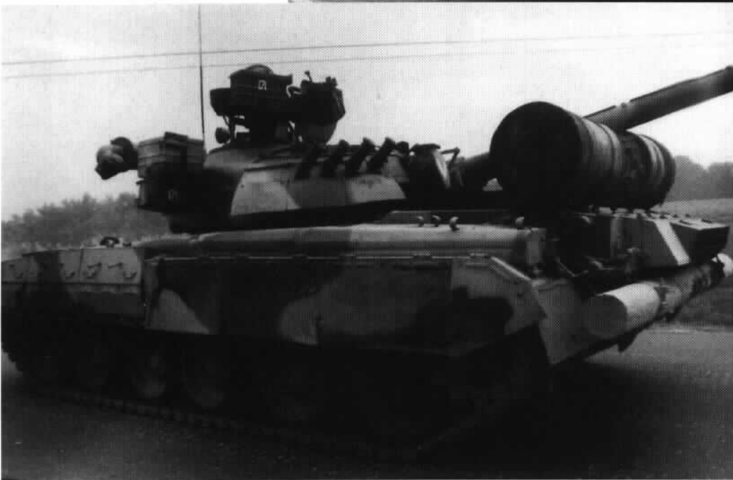
T-80Us on their way to Moscow during the coup. The vehicles have the fuel tanks stowed up on the rear engine deck instead of over the rear fenders as is more commonly the case with turbine powered T-80Bs. (Dr. Udo Bauer Via Thomas Anderson)
