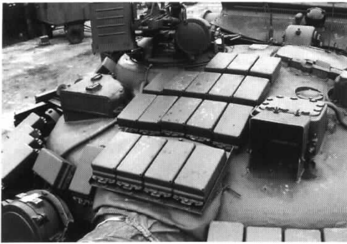
A detail view of the reactive armor array on the roof of the T-80BV as well as the Kobra missile guidance box in front of the commander's station. Note that the bricks on the gun mantlet are contained in a sheet-metal tray. (Michael Jerchel)
