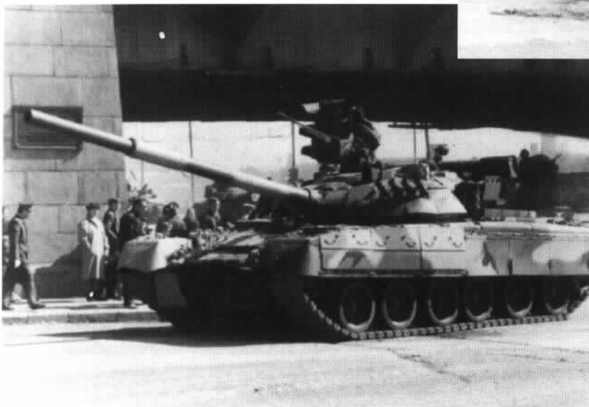
Another distinguishing feature of the T-80U is the rubberized flaps hanging off the turret ERA to give additional stand-off protection.
