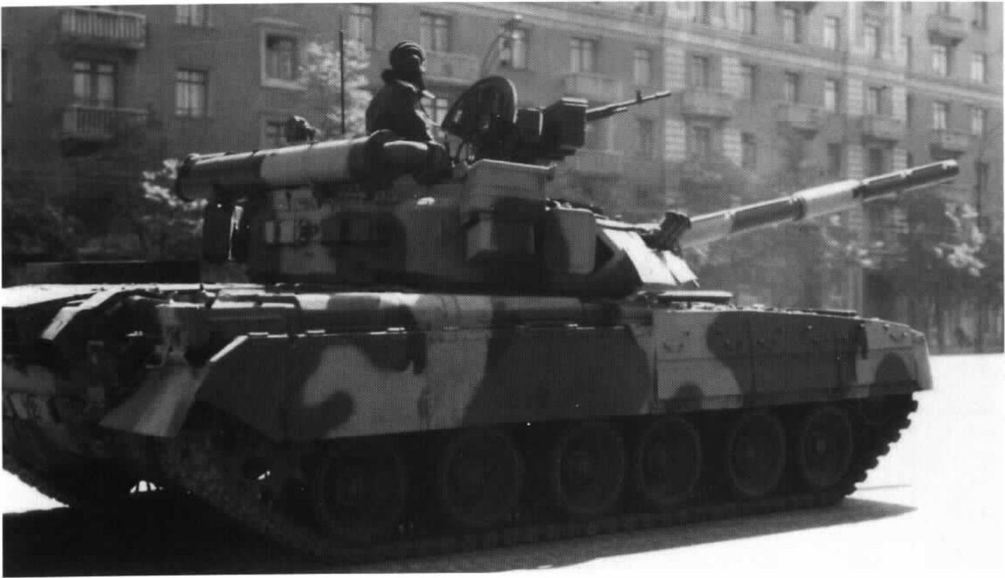
Another side view of the T-80U moving into position in Moscow for a Kremlin parade. The T-80U is not fitted with the usual rear stowage bracket for the OPVT snorkel seen on the earlier T-80B.
