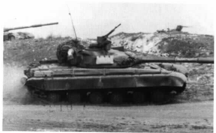
A T-64B on exercise in Hungary in 1989. The small attachment point for the Kobra guided missile control box is evident in front of the commander's cupola.
