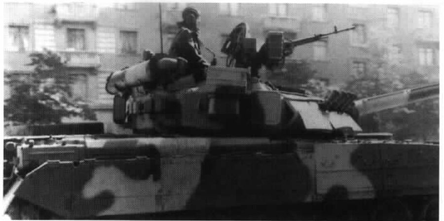
A close-up of the active infrared searchlight on the T-80U. Surprisingly, Soviet tanks still are not fitted with thermal imaging night sights comparable to those used on NATO tanks like M1 Abrams or Leopard II.
