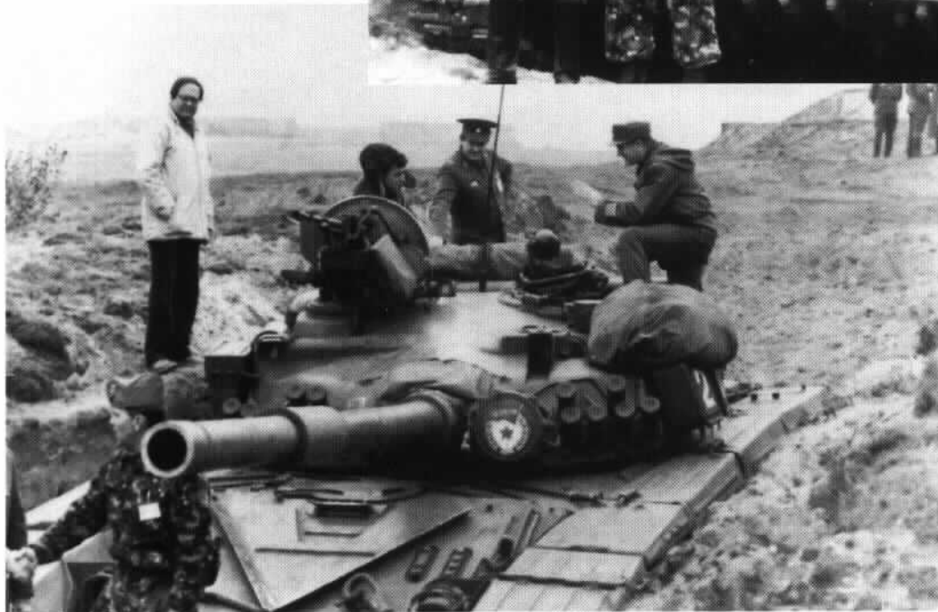
A T-64A rebuild tank crew talking to NATO observers during 1989 wargames in Hungary. Notice how the added glacis armor has cut-out for the KMT mine roller attachments on the hull front outside the V-splash shield.
