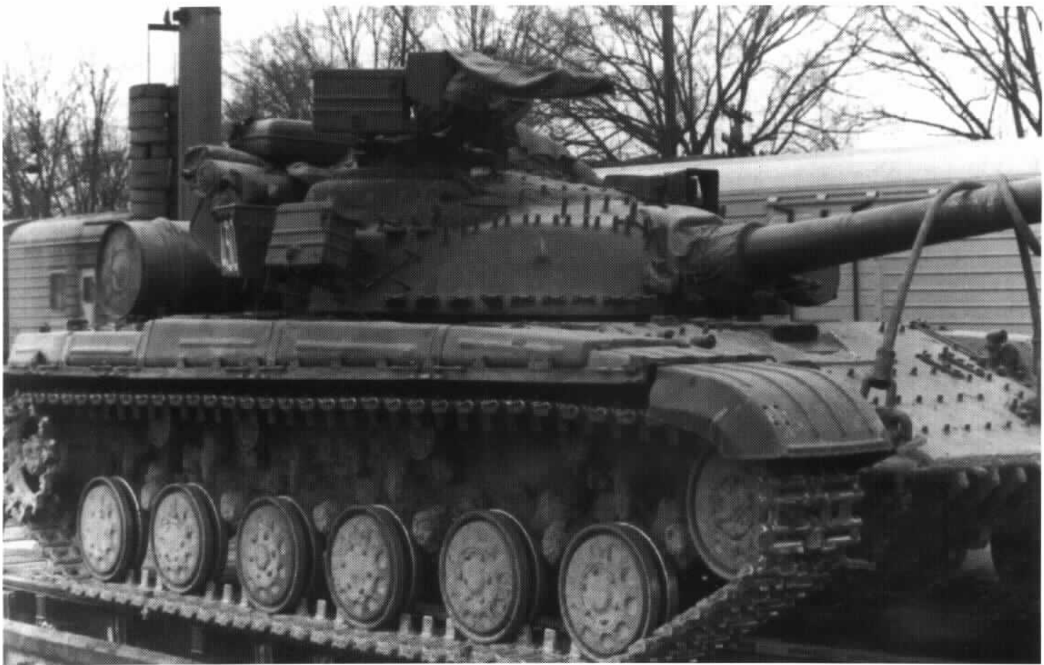
A T-64BV in transit showing the attachment points for the ERA bricks.
