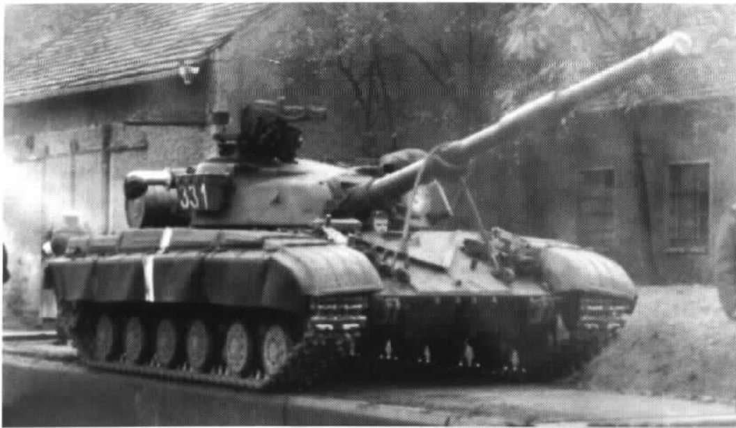
A T-64A rebuild moving off a railroad car during 1989 wargames. This tank is from a Guards unit simulating an aggressor force judging from the white identification band.
