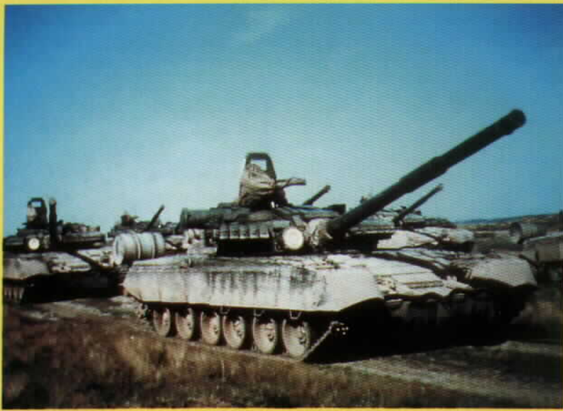
A T-80BV unit on summer maneuvers in the late 1980s. The vehicles are marked with a Guards divisional insignia over a white disc on the active infrared searchlight.
