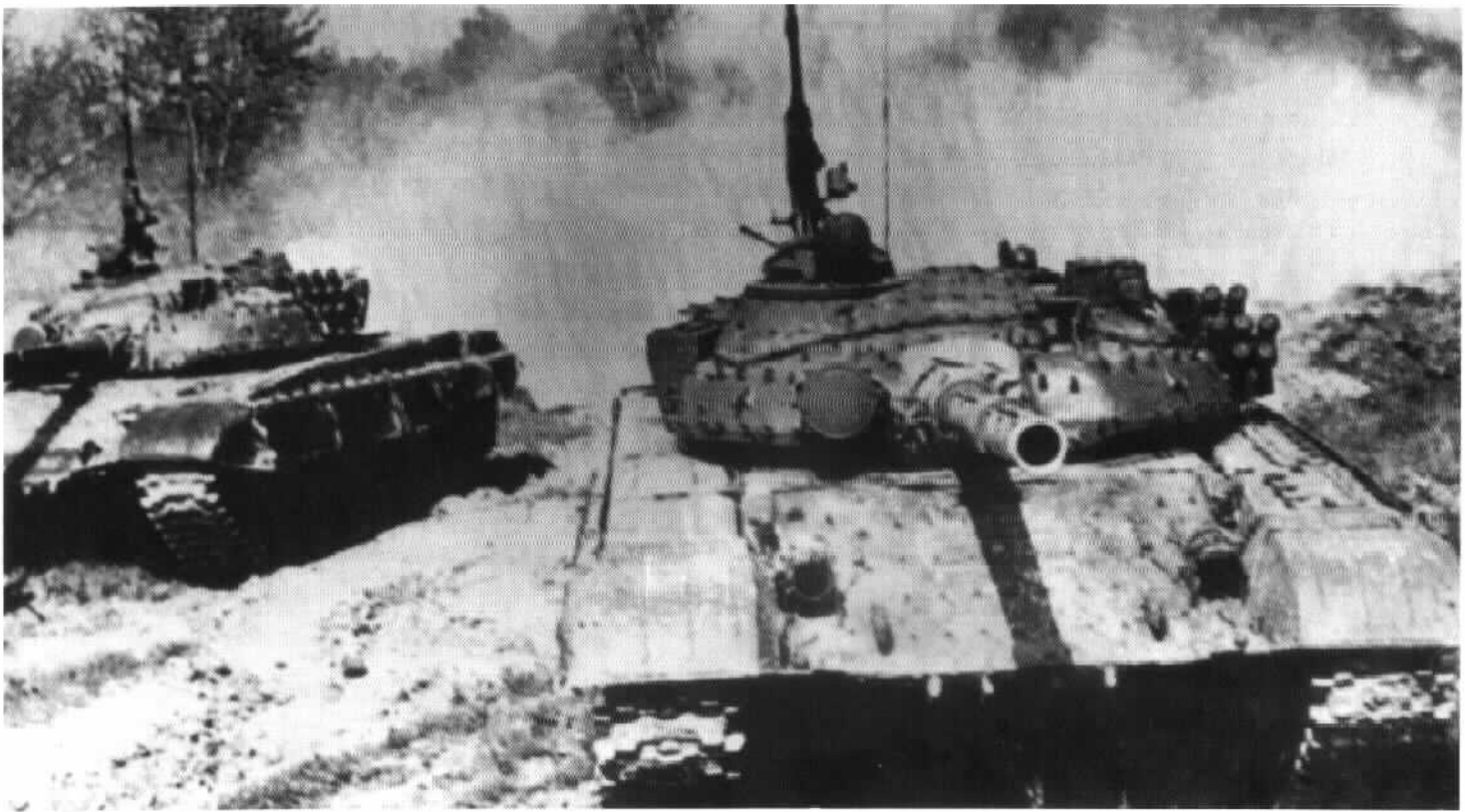
In 1986, the T-72B began showing up with a new gunner's sight immediately in front of the gunner's hatch designated T-72B1. This is a modified version of the 1K13 laser guidance sight and is used with the new 9K120 Svir tube-launched guided missile.
