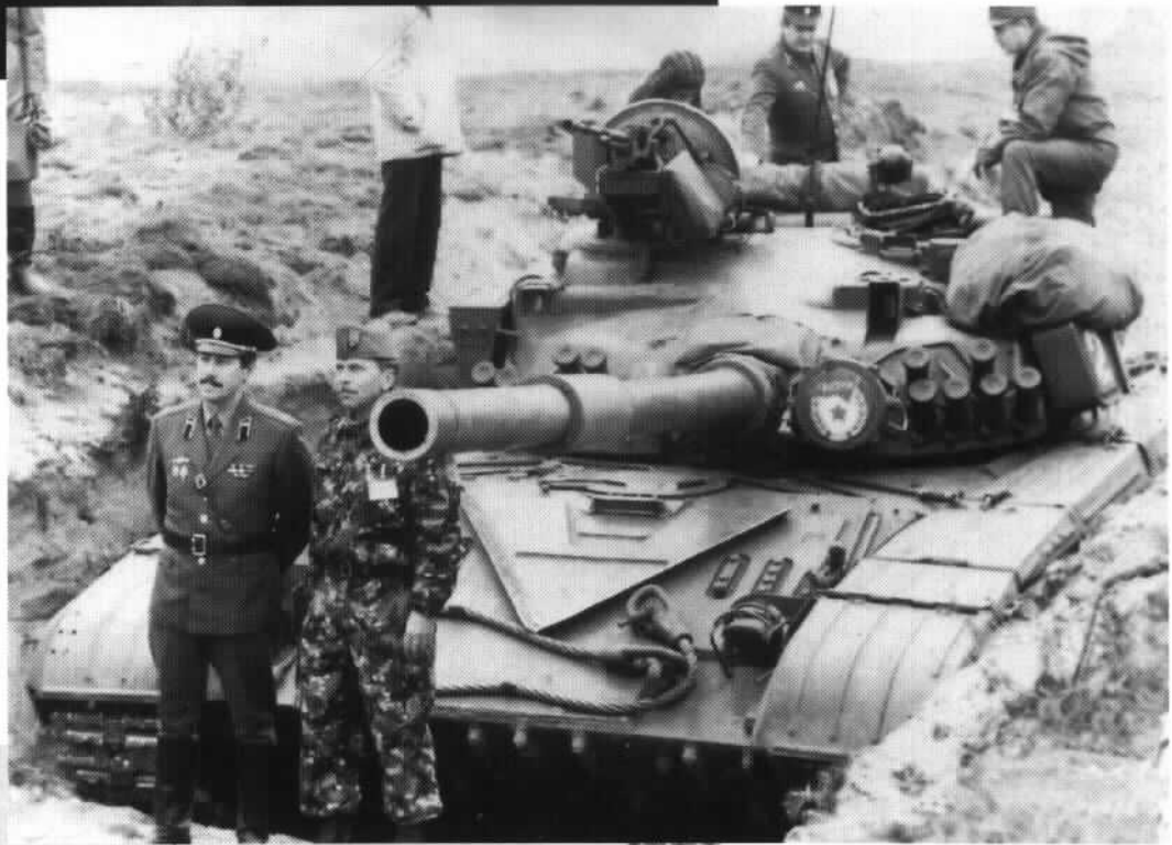
A T-64A rebuild during wargames in Hungary in 1989. This vehicle not only has the basic rebuild features such as the added glacis armor, but also the 12 smoke mortars. In front of the tank is a Soviet officer (to the left, and a Hungarian officer (in camouflage coveralls) to the right.
