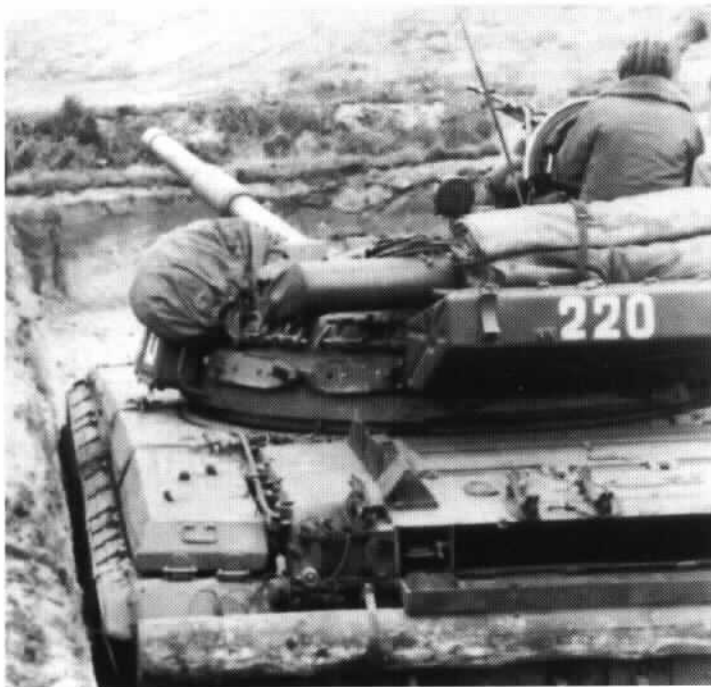
A rear view of a T-64B engine deck. The vehicle is heavily stowed, and is fitted with four racks for spare track links on the left rear turret side.
