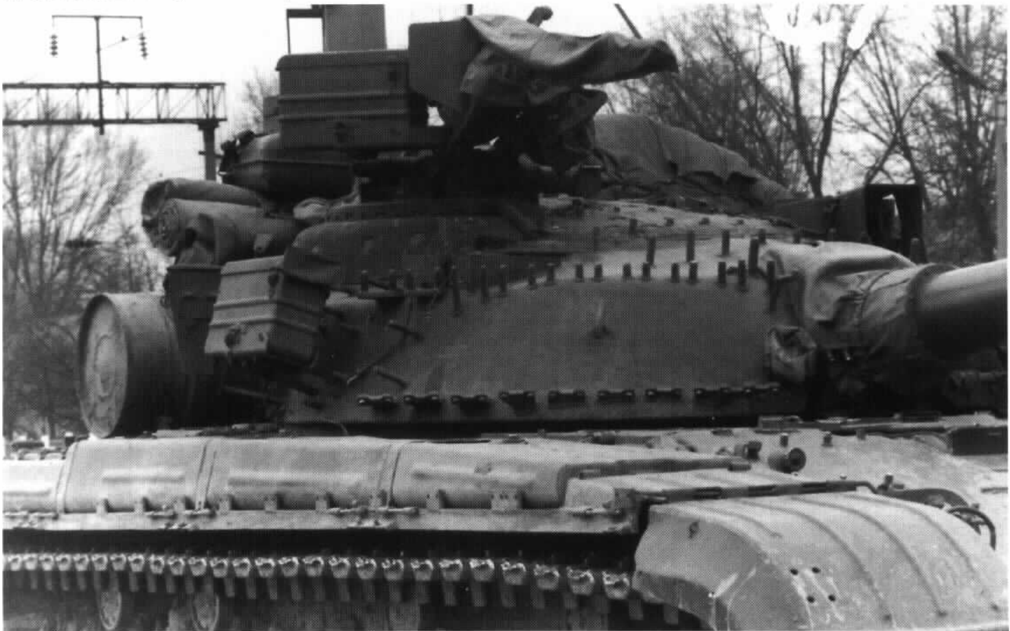
A close-up view of the T-64BV turret minus the bricks themselves. Another detail evident here is the modified attachment arrangement for the Kobra control box, consisted of sheet metal supports under the box. Also evident by careful inspection of this view is the plastic anti-radiation armor on the roof, and around the base of the commander's cupola.
