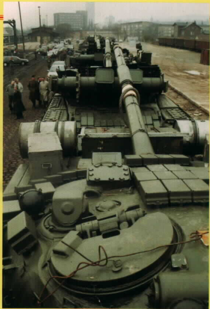
An overhead shot of a T-80BV showing the tank gunner's hatch and the detail in front of it. (Michael Jerchel)
