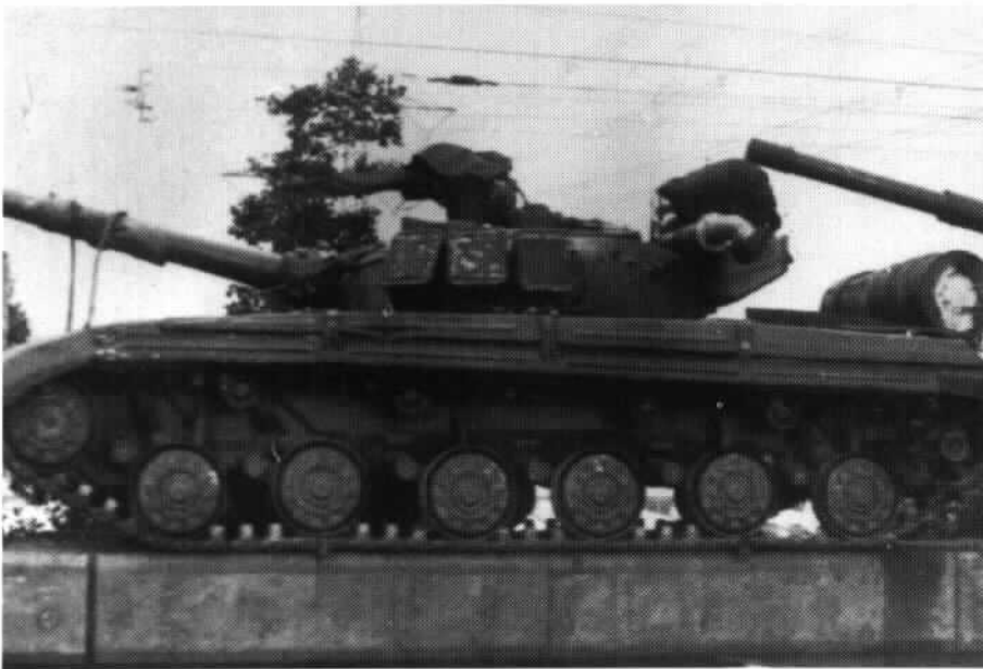
This view of a T-64A in transit gives an unusually clear view of the complicated suspension of the T-64 tank family.
