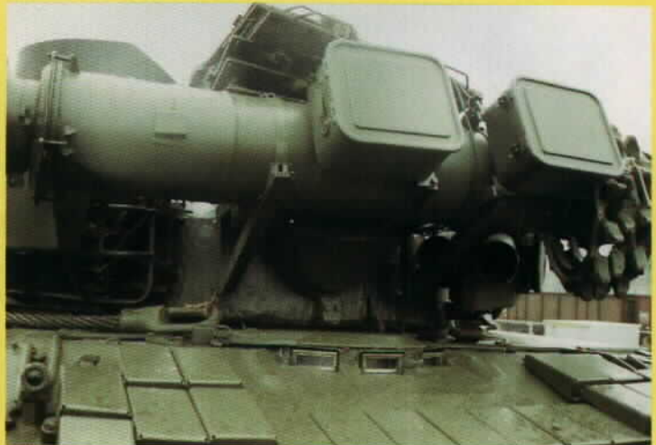
A detail view of the rear turret stowage of a T-80BV. The basic item is the snorkel tube for deep wading. Between the snorkel tube and the turret rear is a combing for the attachment of the snorkeling equipment. (Michael Jerchel)
