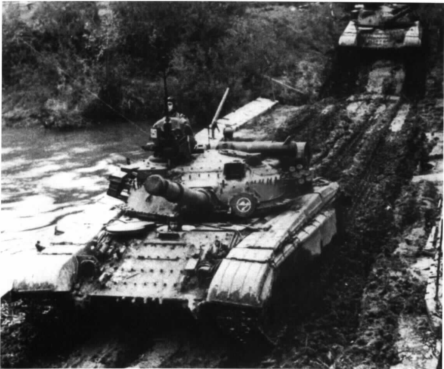
A T-64BV, minus the explosive bricks on summer maneuvers. The many small attachment bolts are very evident in this view. Notice also that the stowage bins and smoke mortar layout has been changed to accommodate the ERA.
