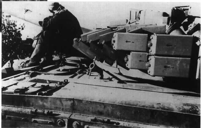
A close-up shot of the ERA bricks on the T-80BV. The marking painted on the brick covers has an arrow pointing forward and the Cyrillic letter "Z" (resembling the number 3) which means Zapad (forward).
